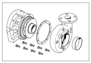
B. Casing, Gasket, and Wearing Ring Removed.
